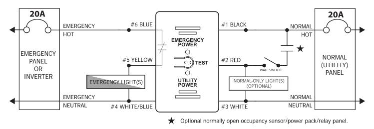
**Wiring Diagram #2 (Shunt):** A dedicated switch controls emergency lighting in a space. Upon loss of normal power, the emergency lighting comes on regardless of switch position.
