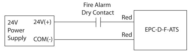
Note: EPC-D-F-ATS red wires are polarity independent
