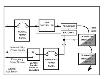
Wiring Diagram #1 (Suggested): During normal operation, the DMX controller
