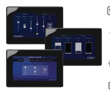
Fresco manages lighting for today's architectural spaces, putting the user confidently in control. Distinguished by its visual appeal and cognitive design, Fresco directly incorporates nLight® devices and controls traditional light sources, LED, RGB and tunable white. Built-in Bluetooth® wireless technology connects with handheld devices. Fresco Touchscreen integrates with building management systems (BMS) through BACnet/IP to trigger scenes and set levels for zones, channels and groups.
